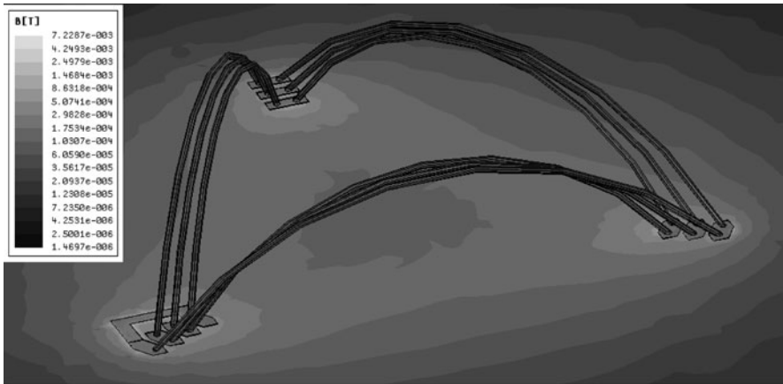
Fig. 3.12 Finite element simulation results. Spatial magnetic field distribution on silicon surface
